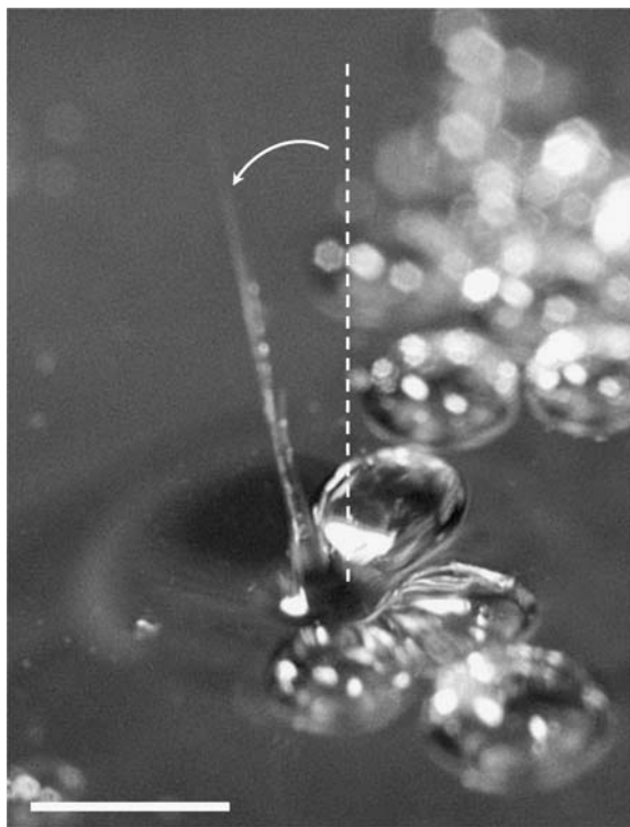
Fig. 38 The liquid-jet deviates from vertical as the neighbouring bubbles' symmetry is broken around a collapsing bubble (bar = 1 mm). (Photograph by Gérard Liger-Belair.)
