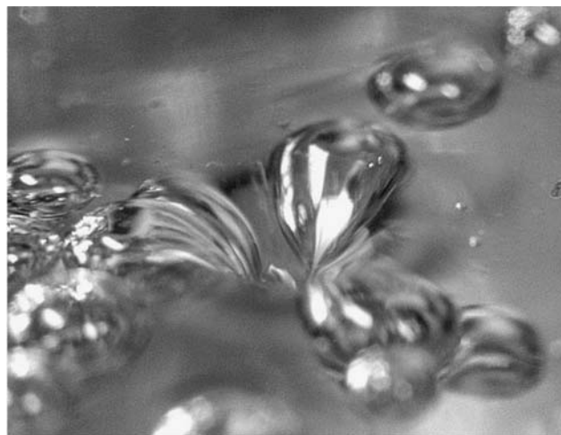
Fig. 35 Shear stresses experienced by bubbles adjacent to a collapsing one at the free surface of a flute poured with champagne (bar = 1 mm). (Photograph by Gérard Liger-Belair.)
