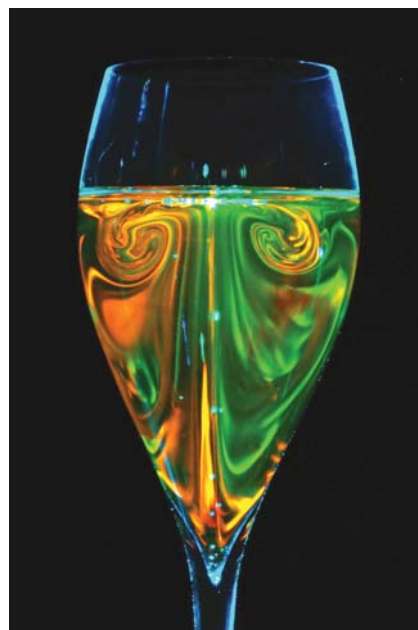
Fig. 27 Flow patterns found inside an engraved champagne flute as highlighted by use of fluorescent dyes injected in the flute section crossed by the laser sheet: sulforhodamine (left), and fluorescein (right). (Photograph by G. Liger-Belair, F. Beaumont and G. Polidori.)
